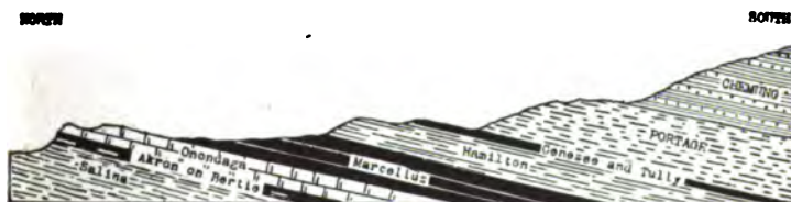
FIG. 1266. — Section (partly on Lake Erie) in western New York, from the head of the Niagara River to the hills of southern New York, showing the succession of the Devonian strata. (Original.)
